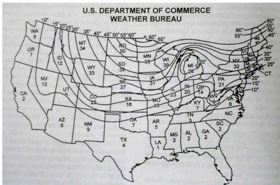
**Figure 6. Average frost penetration depth (in inches)**
